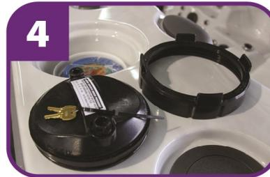
Remove the filter lock ring and lid.
