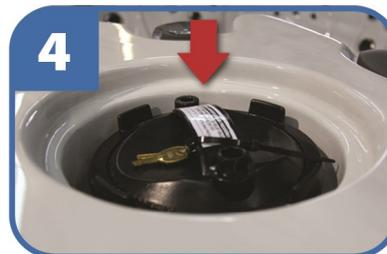
Put filter back into filter canister. Then put back on the filter canister lid and tighten locking ring.
