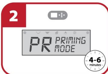
2 PR - Priming Mode: Your spa will now run a diagnostic test. Do not press any buttons while test is running (4 - 6 minutes).
