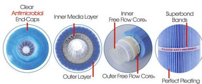
The outer core is similar to a traditional filter which traps larger debris, while the inner core filters the water for particles down to 3 microns in size. The inner core is easily removed and both filter media can be cleaned.
