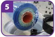
Remove filter and take it out of the plastic transport bag. Leave filter canister open when filling.
