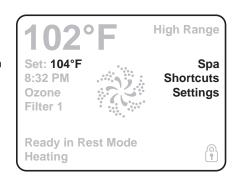
Rest Mode will only allow heating during programmed filter cycles. Since polling does not occur, the temperature display may not show a current temperature until the filtration pump has been running for a minute or two. Ready in Rest Mode may appear when Jets 1 is activated.
