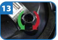
Release any additional trapped air by loosening the air bleed screw. Wait for all air to be released. Retighten.
