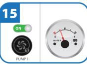
Your water level should read just above 1/4 on the gauge when pump 1 (high speed) is activated. Your hot tub is now filled. Set the temperature and get ready to enjoy!
