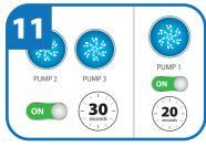
Continue running pumps 2 & 3 (pump 2 on 2-pump models) on high speed for 30 seconds and activate pump 1 on high speed for 20 seconds.
