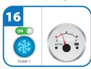
Your water level should read just above 1/4 full on the gauge when pump 1 (high speed) is activated. Your hot tub is now filled. Set the temperature and get ready to enjoy!
